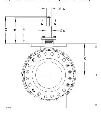
Figure 5. Shaft Detail (see table 3)
