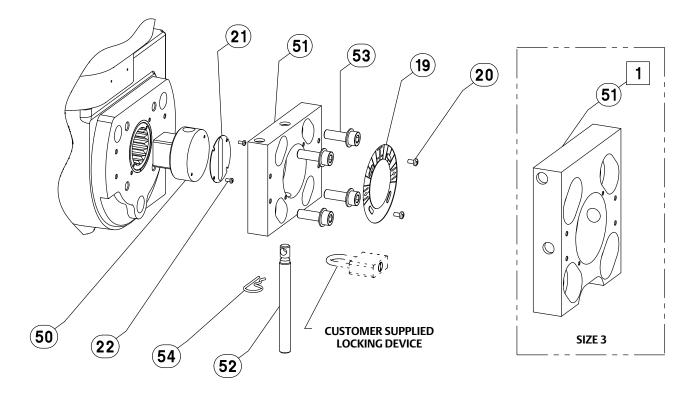
PART ORIENTATION FOR SIZE 3 END-MOUNT INSTRUMENT
