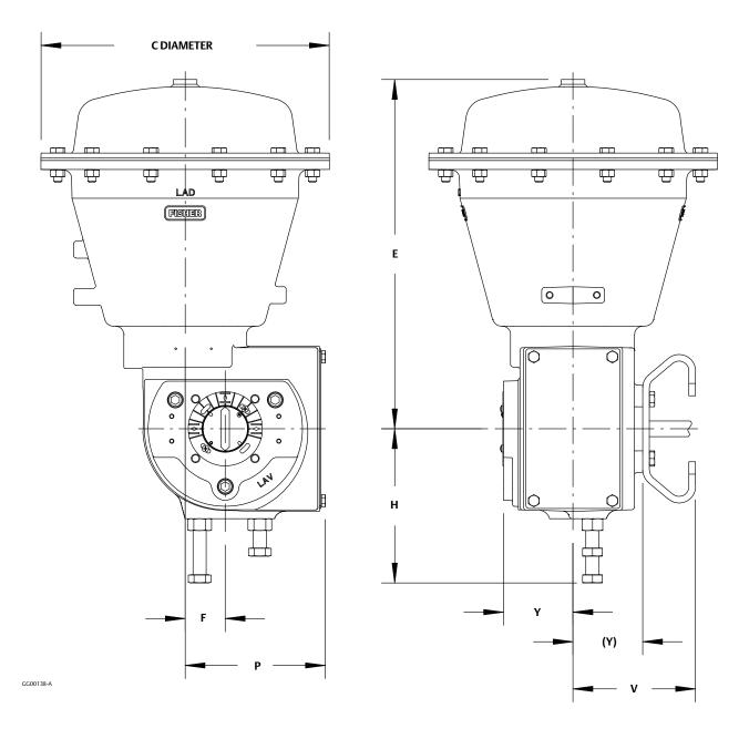
Figure 4. Handwheel Dimensions (also see tables 6 and 9)
