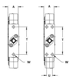
Figure 9. Dimensions for Fisher 8580, Wafer Style Valve (limited sizes)
