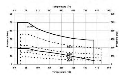
Figure 6. Material Pressure/Temperature Curves
