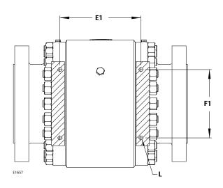
Figure 7. NPS 14 CL600 thru NPS 24 CL600 Base Bracket Dimensions (see table 3)
