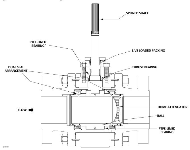
Figure 2. Construction Versatility Seal/Dome Assembly Details
