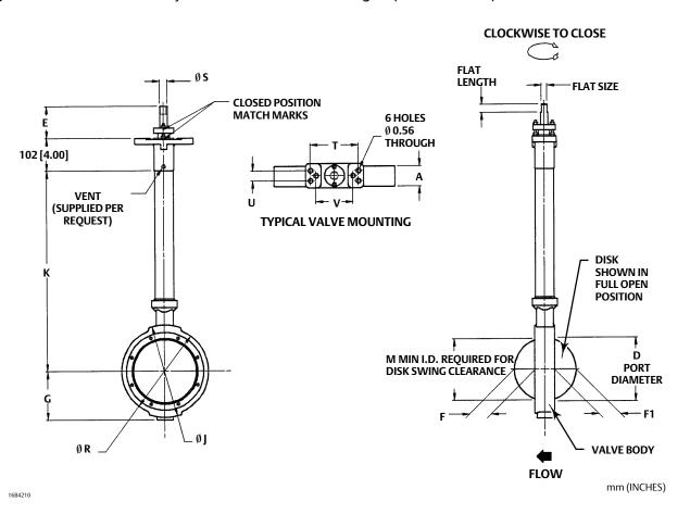
Table 4. Dimensions, Single Flange Style Valves, CL150, NPS 3 through 8
