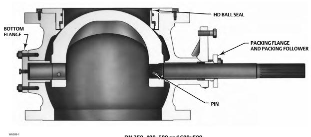
DN 350, 400, 500 and 600x500 (NPS 14, 16, 20, and 24x20) VALVES (HD BALL SEAL)
