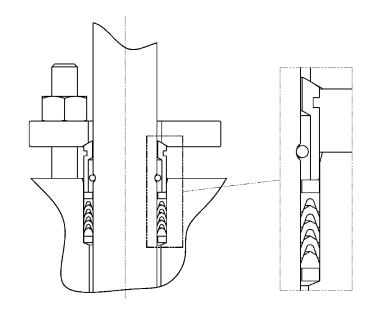
NPS 3 THROUGH 8 WITH ANTI-BLOWOUT RING
