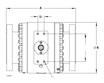
Figure 4. NPS 24 CL600 Packing Box Housing Mounting Pad Dimensions (see table 2)
