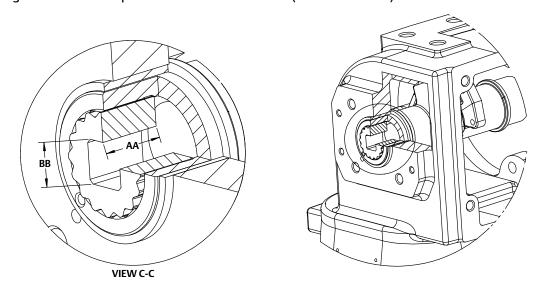
Figure 8. Fisher 2052 Actuator Mounting Styles (also see table 13)
