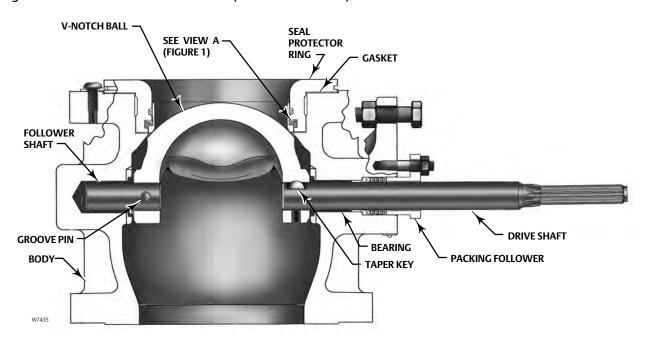
DN 80 THROUGH 300 (NPS 3 THROUGH 12) VALVES (HD BALL SEAL SHOWN)
