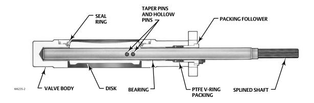
Figure 2. Available Seal Configuration
