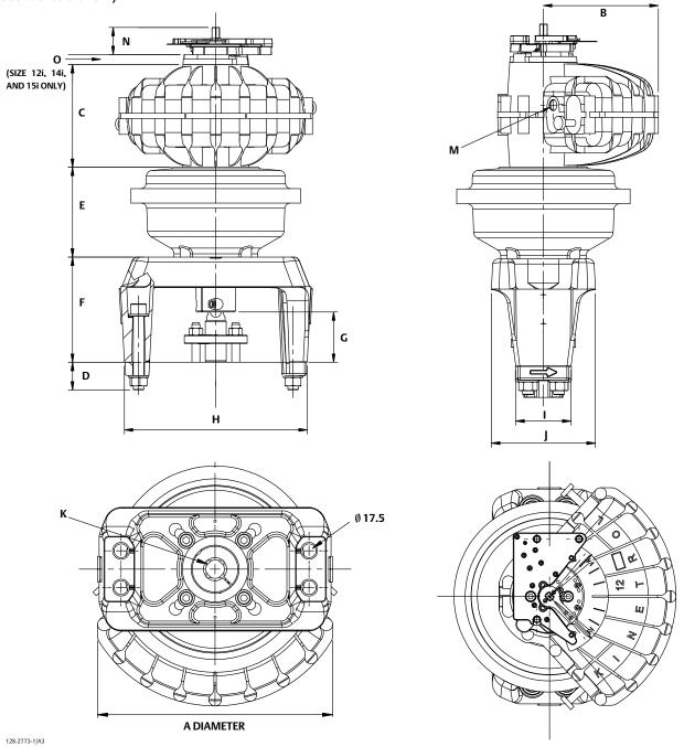
Table 8. Actuator/Valve Body Mounting Dimensions 16 through 30 (see figure 4)
