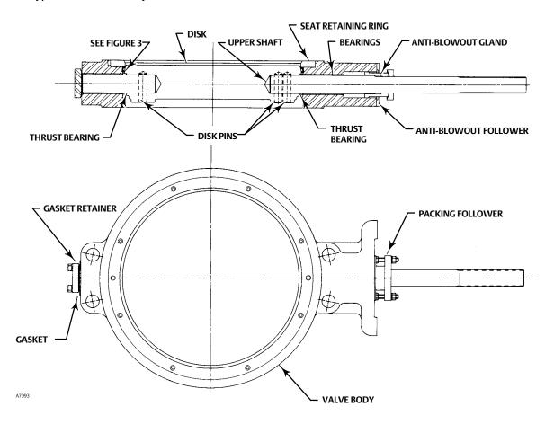
Figure 6. Blowout Protection
