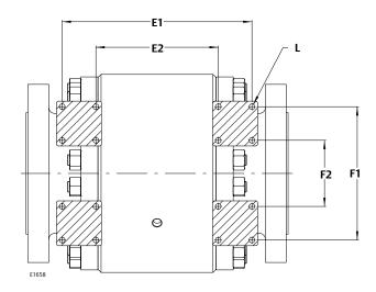
Figure 8. Live-Loaded Packing Arrangement Details
