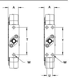
Figure 9. Dimensions for Fisher Control-Disk Valve, Wafer Style (limited sizes)
