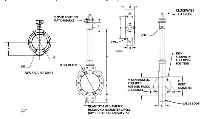
Table 10. Dimensions, Single Flange Style Valve, CL300, NPS 8 through 24
