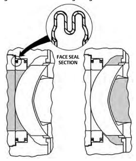
FORWARD FLOW SHUTOFF REVERSE FLOW SHUTOFF 4283375-A
