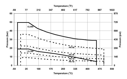
Figure 6. Material Pressure/Temperature Curves
