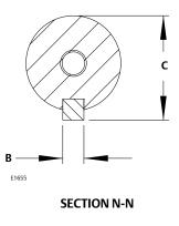
Figure 6. NPS 6 CL600 thru NPS 14 CL300 Base Bracket Dimensions (see table 3)
