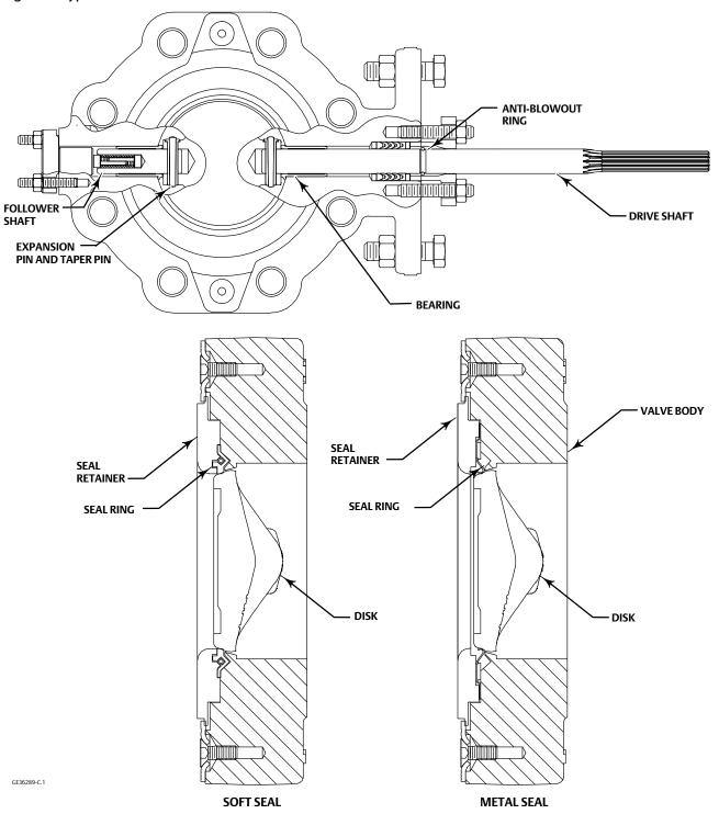
Note: Split shaft construction shown. Size NPS 8 through NPS 12 are thru-shaft.
