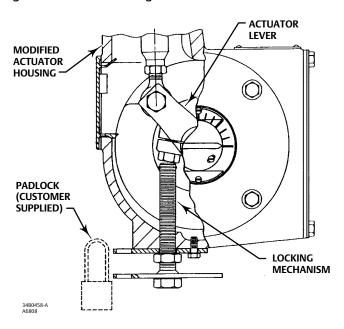
Figure 5. Actuator Locking Mechanism for Size 80 and 100 Actuators
