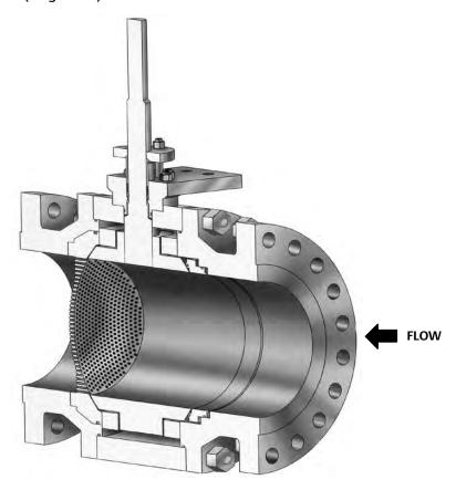
Figure 2. Aerodome and Hydrodome Attenuator Details
