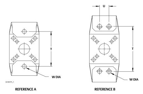
Figure 6. NAMUR Instrument Mounting Dimensions (also see tables 10 and 11)
