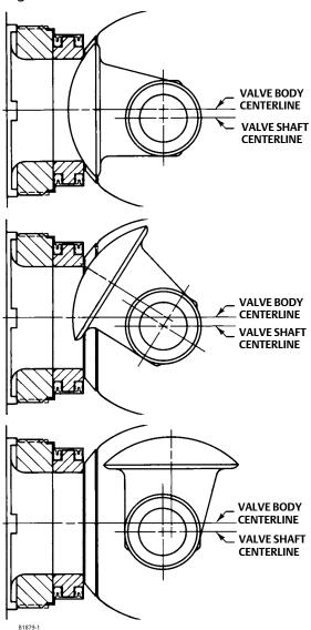
PDTC—Push-down-to-close (extending actuator rod closes valve)
