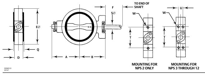
NOTE: FOR NON-CODE MATERIAL THE ASME CLASS REPRESENTS DIMENSIONS NOT PRESSURE TEMPERATURE RATING. DISK CHORDAL SWING DIA. AT VALVE FACE IS "M". PLEASE VERIFY CLEARANCE WITH PIPING.
