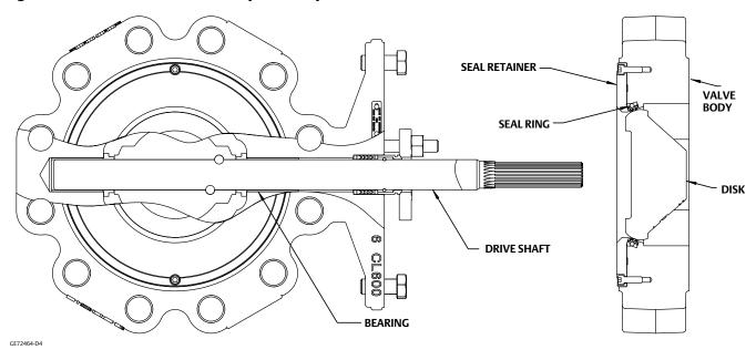
Figure 3. 8590, NPS 8 to 24, Valve Body Assembly 🗇
